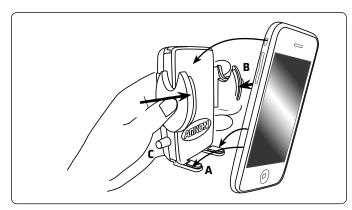
Push the release button (C) to open the side grip arms and remove the device.
